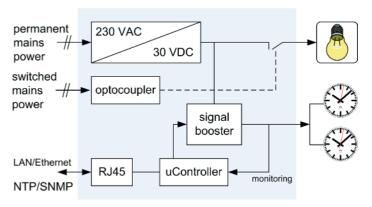
Network clock, fully PoE powered (illumination control by switched mains power)
